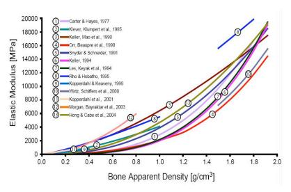
elastic modulus in the litterature (see plot). VA-BATTS is using the Keller 1994 relation but users may want to select a different one. Once the elastic modulus image is created another relation is used to create a shear modulus [MPa] image (A\_G). VA-BATTS is using the Reilly & Burstein 1976 relation but users may want to select a different one.
