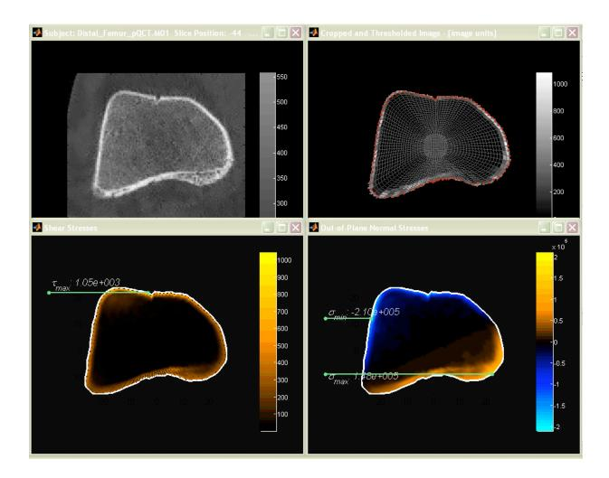
The program also reports the sectional properties such as the moments of inertia etc. but also calculates and prints the Torque that the cross section is supporting. The user is advised to look into the last line of the main.m routine to find out what other metrics are calculated.
