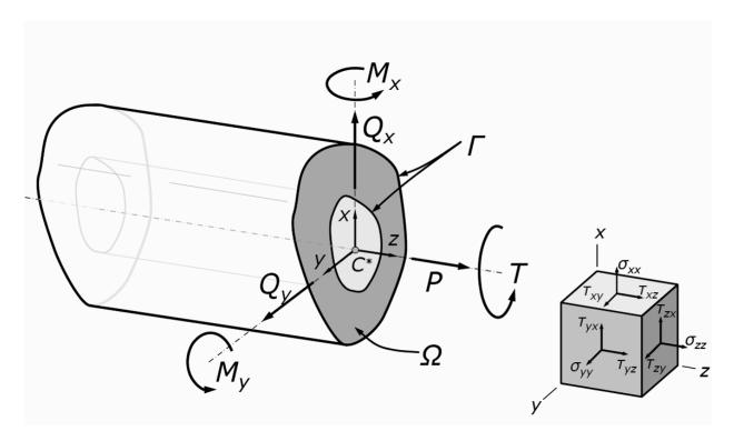
coordinate system of the bone as well as the possible applied loads.
