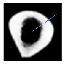
As shown in the plot, the dots represent the pixel values across the search zone. The graph represents a fit of those data points by the cumulative (error) function. This function is described in fun.m
