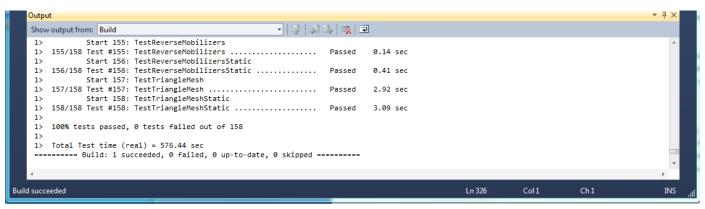
The complete set of 158 dynamic and static regression tests using debug libraries ran in about 10 minutes on my i7 machine (closer to 1 minute for release libraries).
