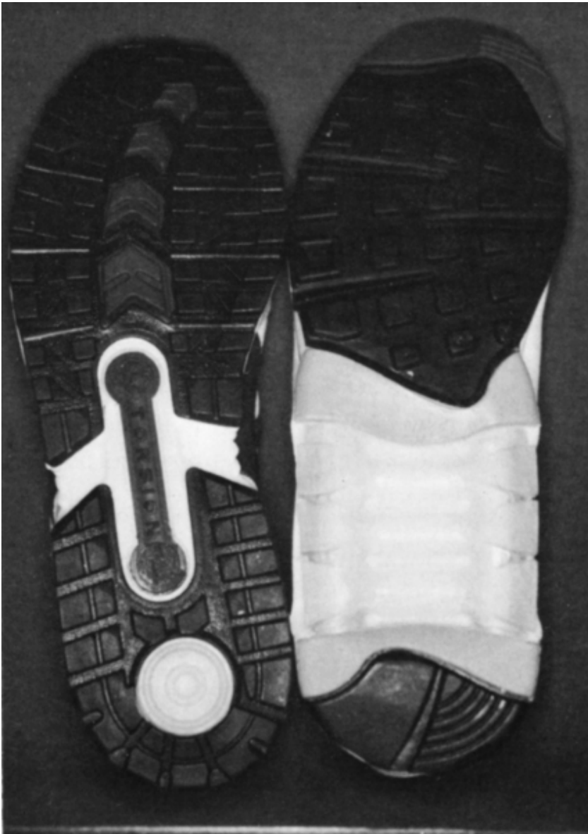
Figure 25B-26 Example of wide versus narrow midsole widths used in the Nike ( right ) and Adidas ( left ) running shoes. (Photograph by Thomas O. Clanton.)
