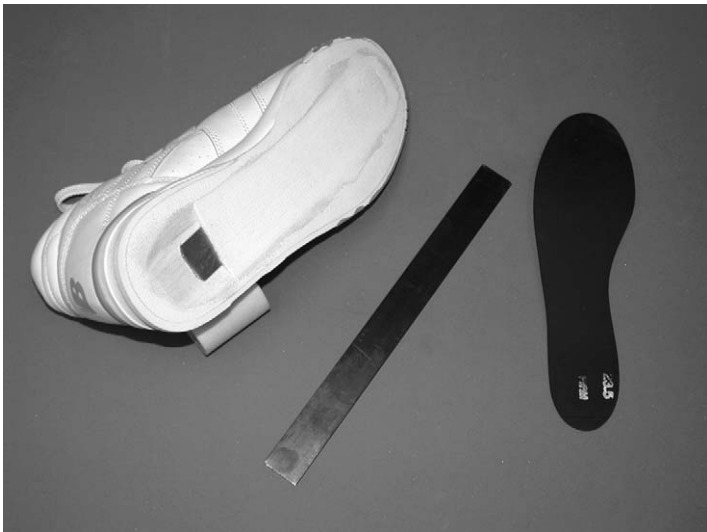
Fig. 1. Shoe with extended steel shank and an example of a carbon fiber plate.
