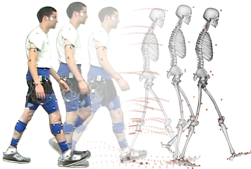
Figure 2-1: Inverse Kinematics Tool Overview. Experimental markers are matched by model markers throughout the motion by varying the generalized coordinates (e.g., joint angles) through time.
