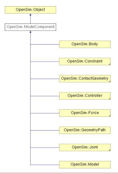
The classes that implement model components in OpenSim all derive from a single base ModelComponent class: implements createSystem()
