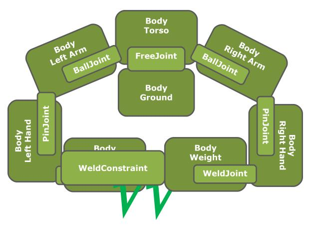
Constraint is required to form a closed loop
