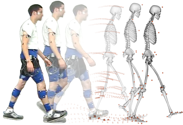
Figure 2-4: Inverse Kinematics Tool Overview. Experimental markers are matched by model markers throughout the motion by varying the generalized coordinates (e.g., joint angles) through time.
