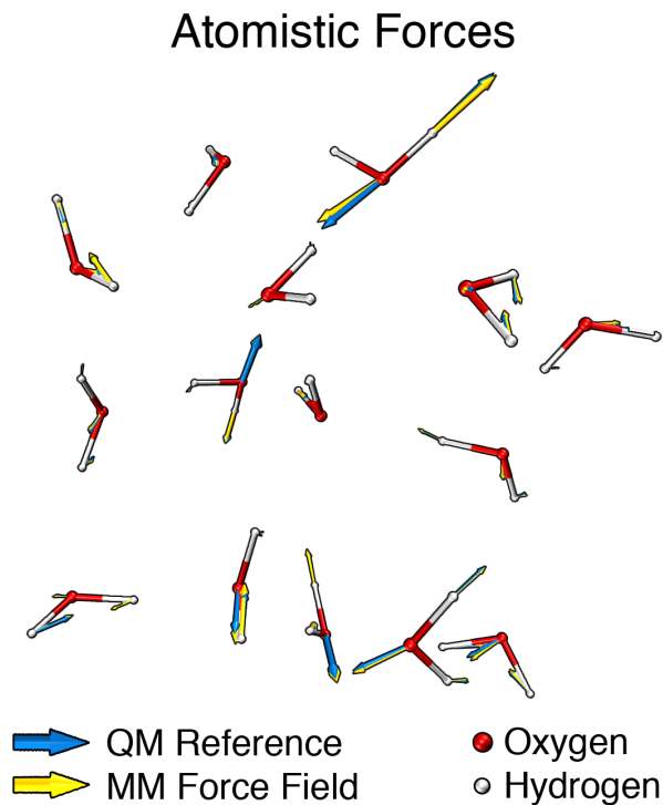
Figure 5: Atomistic forces on a representative water 15-mer from the QM reference data (blue) and the force field (yellow), showing near-coincidence for many atoms. The representative configuration demonstrates a force field with a RMS force error of 11%. The lengths and thicknesses of the force vectors were scaled by an arbitrary global factor to aid visualization.
