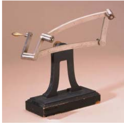
Figure 6: a mechanism with four joints; at most three can be mobilizers
