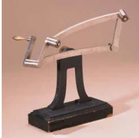
Figure 3: a mechanism with four joints; at most three can be mobilizers
