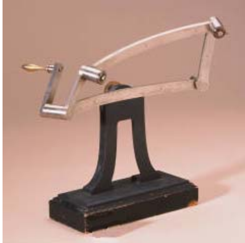
Figure 8: a mechanism with four joints; at most three can be mobilizers
